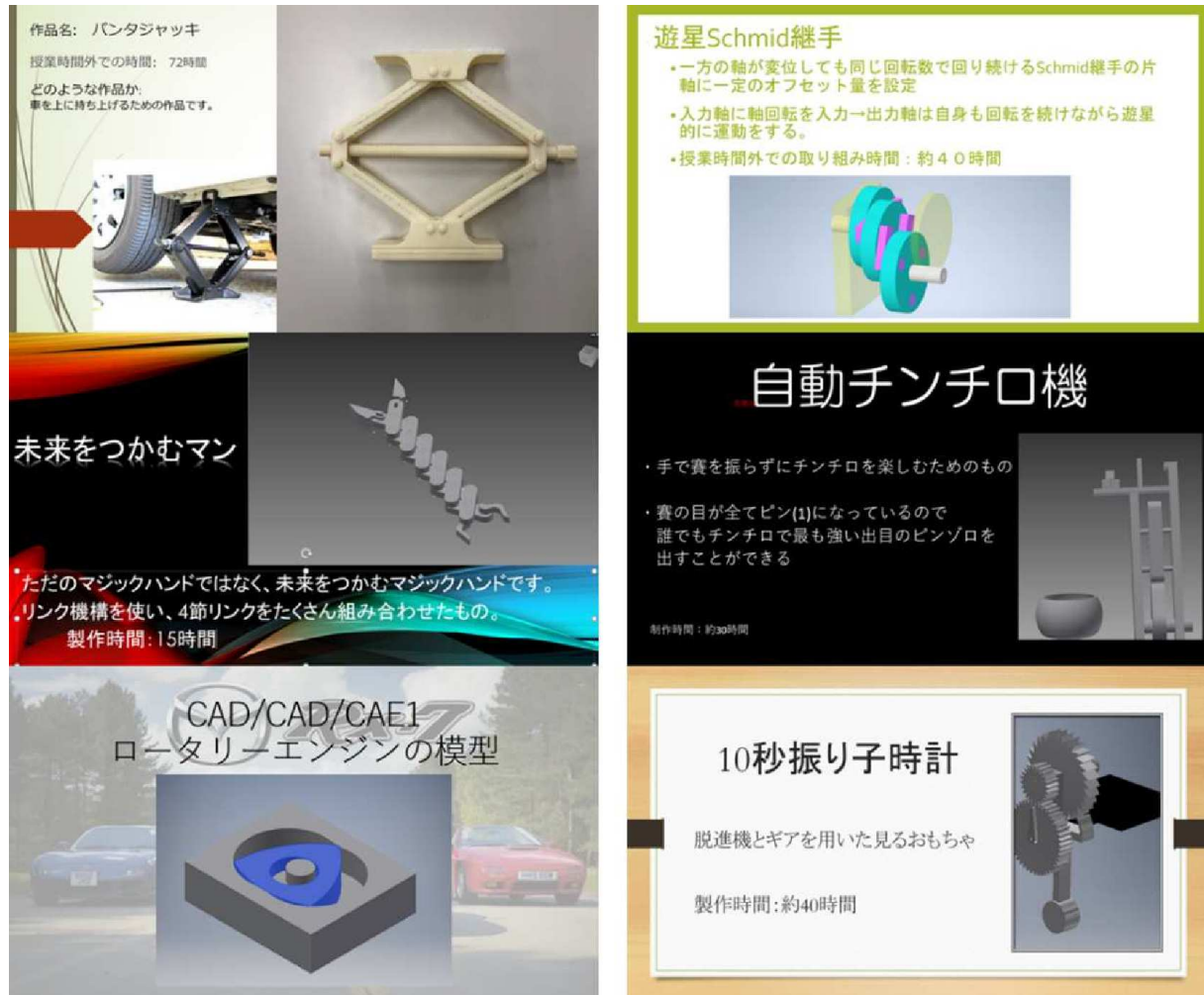
FIGURE 3. Examples of students' works presented in the 15th session. The upper left work is a pantjack, which took 72 hours of work outside of class time. The work on the left in the middle row is a magic hand, which took 15 hours to make. The work on the left in the lower row is a model of a rotary engine. The upper right work is a planetary schmid joint, which took approximately 40 hours of work outside of class time. The work on the right in the middle row is an automatic dice-rolling machine, which took approximately 30 hours to make. The work on the lower right is a 10-second pendulum clock, which took approximately 40 hours to make.
