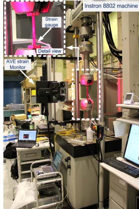
Fig. 12 Tensile test setup.
