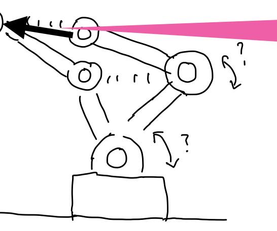
Path planning problem: verify if the end-effector can be moved along the given path → calculate a series of corresponding algles of the joints
