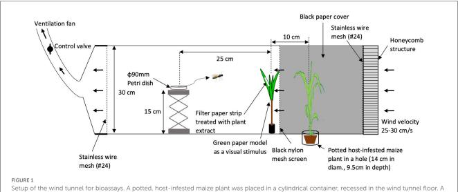
Setup of the Wind tunnel for bioassays. A potted, nost-infested maize plant was placed in a cylindrical container, recessed in the Wind tunnel floor. A honeycombed diffuser panel was fixed at the windward end of the tunnel to facilitate laminar airflow. Stainless wire mesh screens at both end sides of the wind tunnel were equipped to avoid escapes of wasps. Arrows indicate the direction of airflow. In Experiment 1, the filter paper strip was attached directly to the green paper model.
