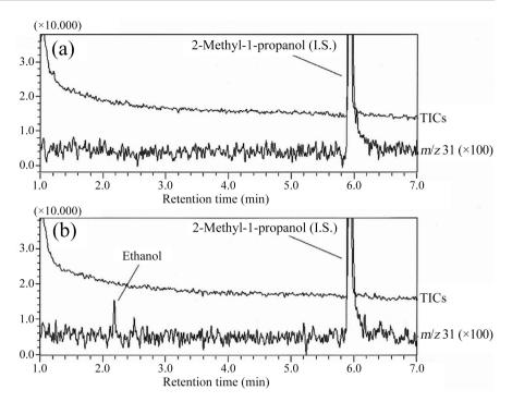
**Figure 2.** Total ion current chromatograms (TICs) and extracted ion chromatograms (EICs) obtained from (a) one of 80 blood specimens (ethanol was not detected) and (b) the blank blood specimen spiked with ethanol (concentration: 0.001 mg/mL).
