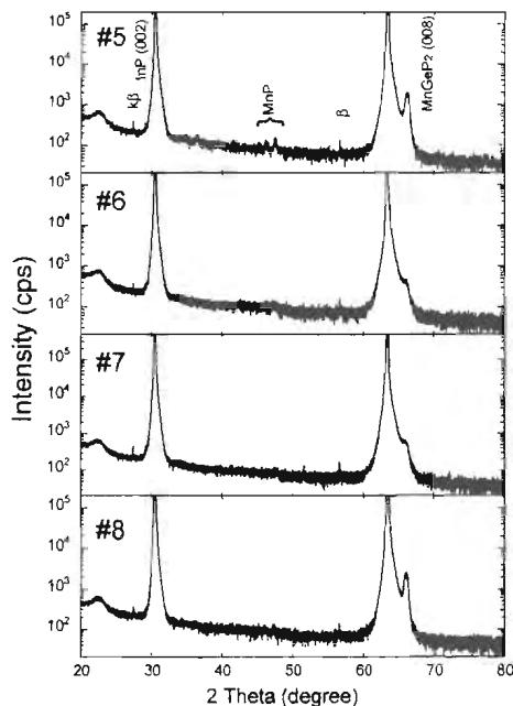
**Fig. 3.** XRD patterns of thin films prepared on InP (001) substrates shown in Table II.
