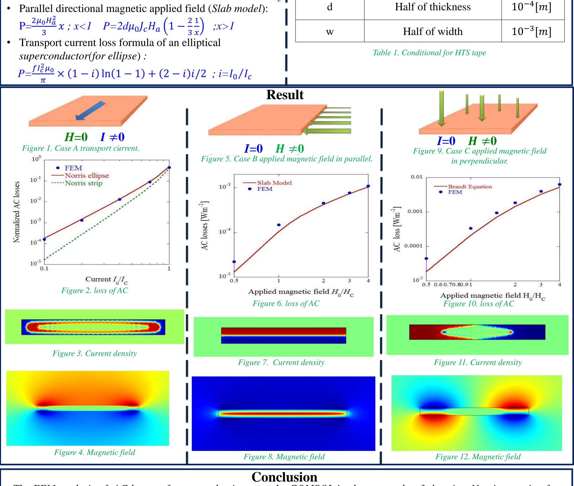
The FEM analysis of AC losses of superconducting tapes by COMSOL is almost equal to 3 theories: Norris equation for ellipse, Brandt equation and Slab model.
