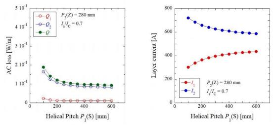
(a) AC loss characteristic against  $P_1(S)$ . (b) Layer current characteristics against  $P_1(S)$ . Fig.4 AC loss and layer current characteristics against  $P_1(S)$  when  $P_2(Z) = 280$  mm.
