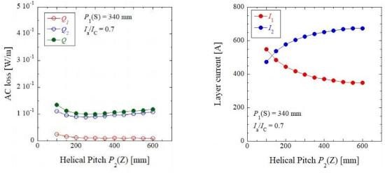
(a) AC loss characteristic against  $P_2(Z)$ . (b) Layer current characteristics against  $P_2(Z)$ . Fig.3 AC loss and layer current characteristics against  $P_2(Z)$  when  $P_1(S) = 340$  mm.
