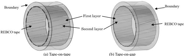
Fig.1 3D model of two-layers REBCO superconducting cable
