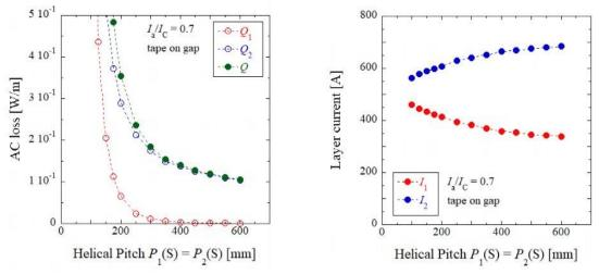
(a) AC loss characteristic against  $P_1(S) = P_2(S)$ . (b) Layer current characteristic against  $P_1(S) = P_2(S)$ . Fig.7 AC loss and layer current characteristics against  $P_1(S) = P_2(S)$ .
