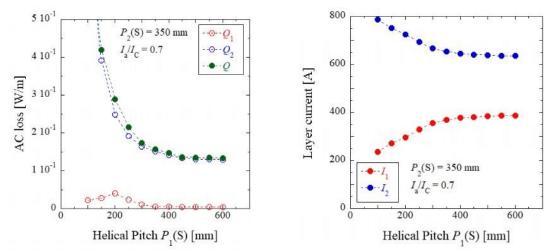
(a) AC loss characteristic against  $P_1(S)$ . Fig.6 AC loss and layer current characteristics against  $P_1(S)$  when  $P_2(S) = 350$  mm.
