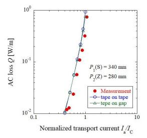
Fig.2 AC loss characteristic against normalized current.
