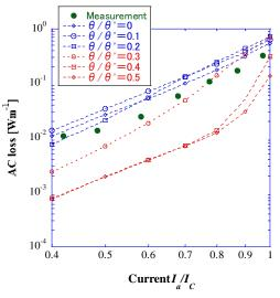
Fig. 6 AC loss characteristics of two layers cable-conductor with relative position angle changed
