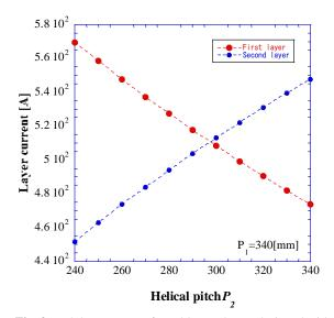
Fig. 9 Each layer current for cable-conductor designed with minimum loss.
