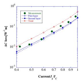
Fig. 4 AC loss characteristics of two layers cable-conductor with uniform layer current.
