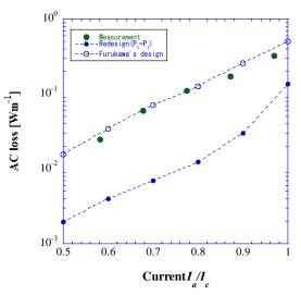
Fig. 10 AC loss characteristics by quasi three-dimensional electromagnetic field analysis.
