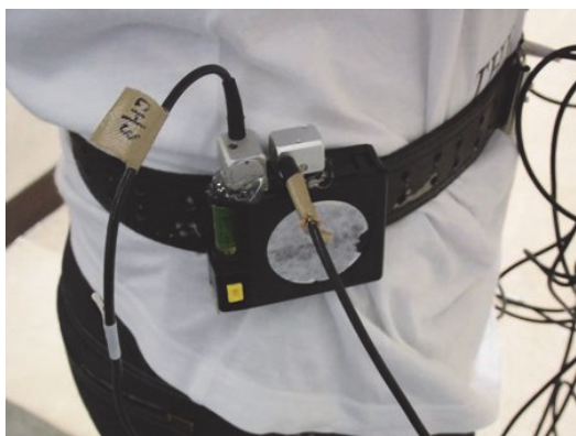
Fig.1 Setup of accelerometers on a person being tested.
