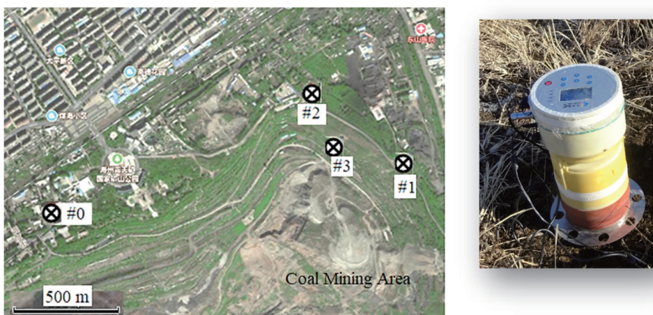
Fig.5 Measurement locations in the coal mining area (Fuxin City, Liaoning Province, China) and the CO 2 flux monitor (point#0: normal area, points #1, 2 and 3: coal mine area) 16) .
