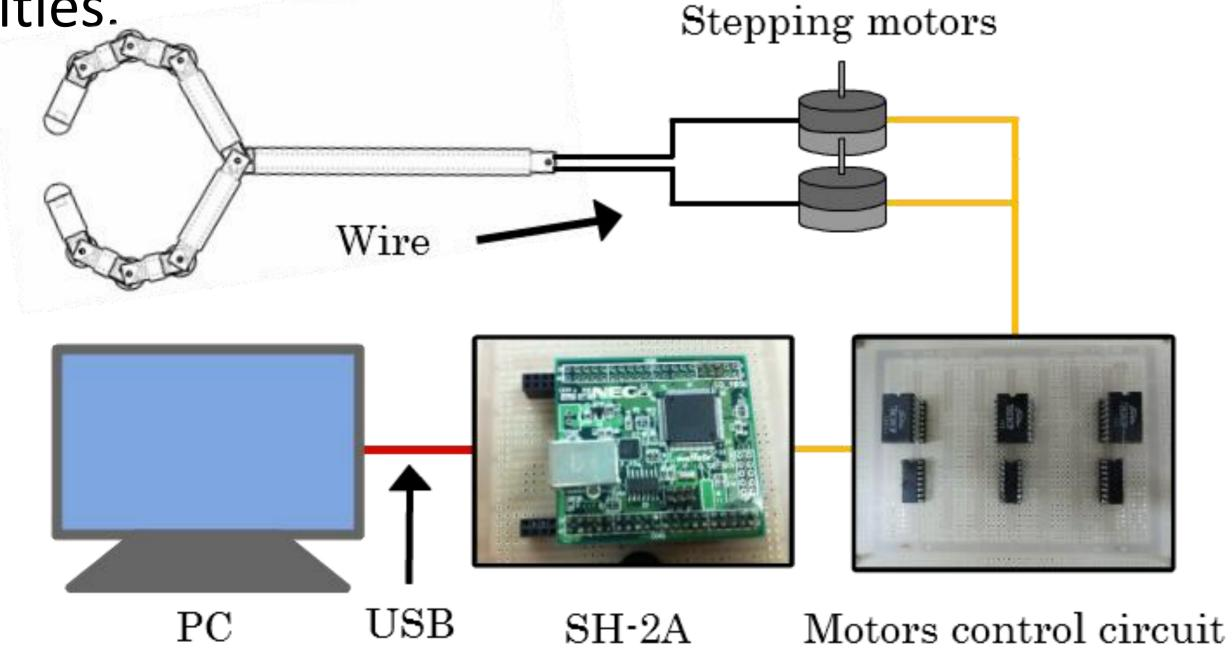
We used a readily available plastic material in order to minimize the weight of the system. Wires were used for operating the fingertips to realize flexible behavior of the robotic hand system. Moreover, such a setup can prevent the positioning error due to gear's backlash. Springs were used for opening and closing the fingers.
