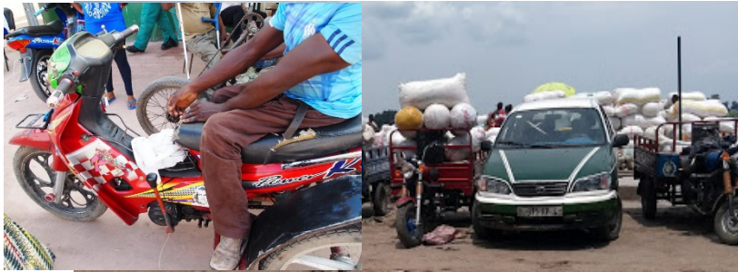
Figure 2. A modified tricycle for PWDs called ‘adaptation’. Gears are changed with the left hand (photographed on 21 November 2013)
