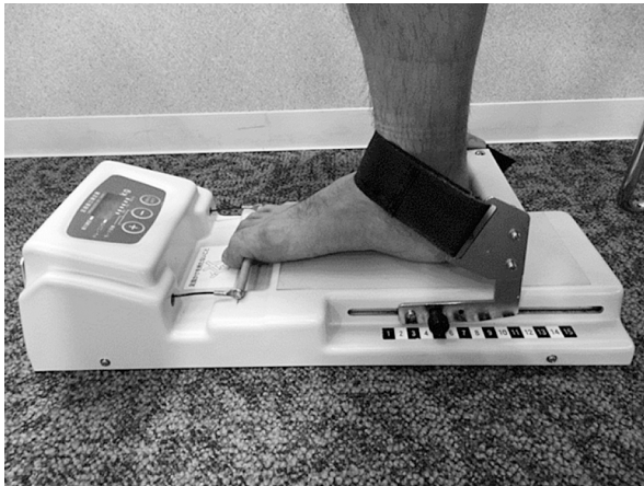
Fig. 1 Measurement of toe flexor strength using a toe grip dynamometer.
