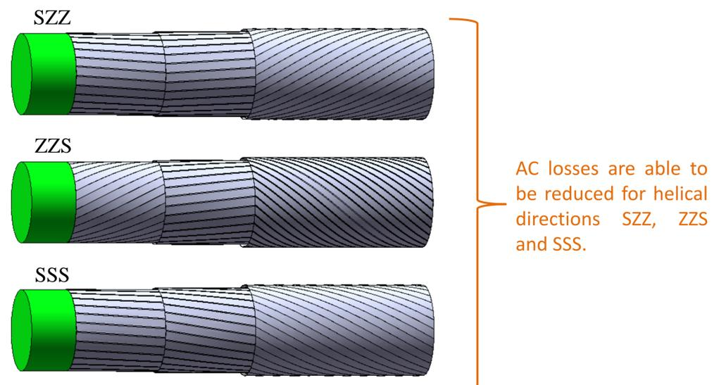
Fig.7 Helical directions of HTS cable conductors
