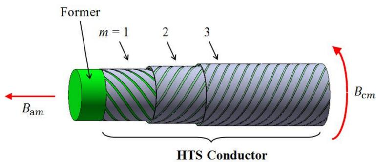
Fig.1 Structure of HTS cable conductor
