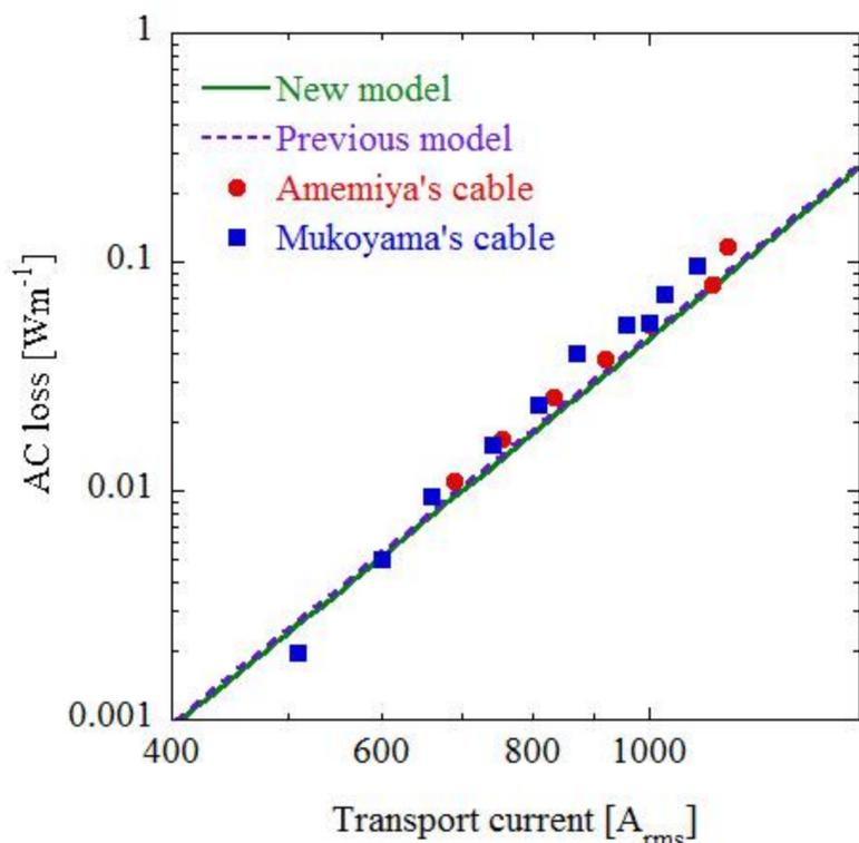
Fig.4 AC losses as a function of transport current for the HTS cable
