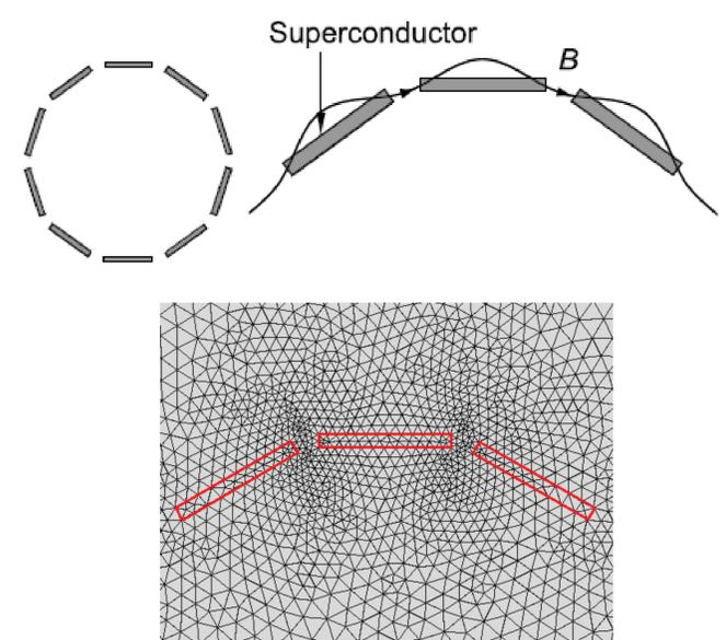
Fig.10 Computation of AC losses by FEM
