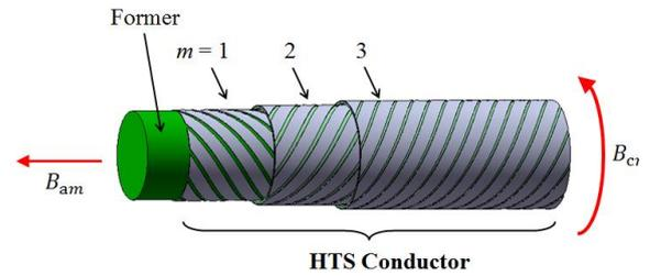
Fig. 1. Structure of the superconducting cable
