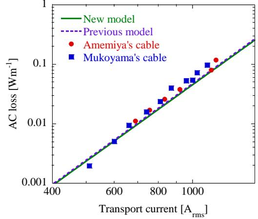
Fig. 4. The AC loss of the transmission currents
