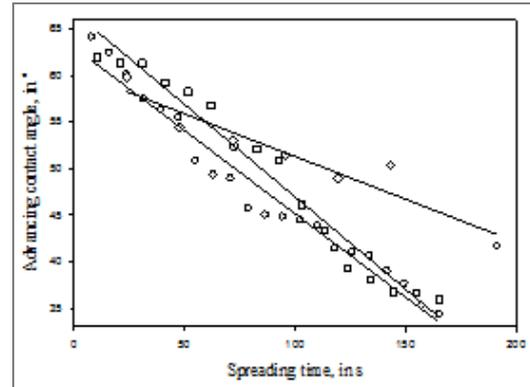
**Fig.2.** Dynamic contact angles of different solution brines (○) B1; (□) B2; (◇) B4
