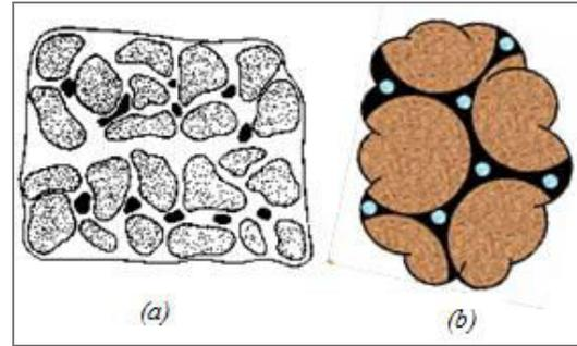
**Fig.1.** Schematic of water-wet rock (a) and oil-wet core (b); Modified from reference [5]
