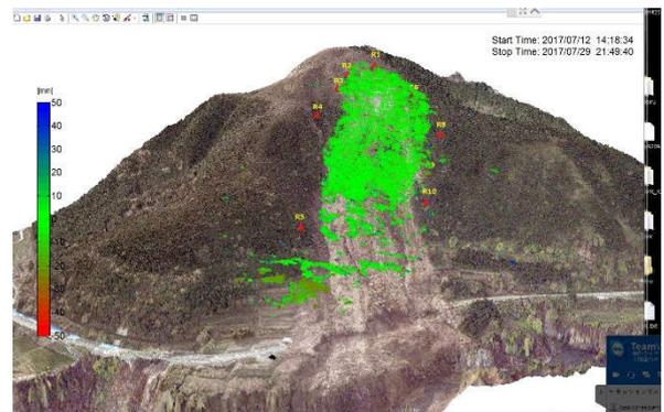
Fig. 2. GB-SAR Interferometry at Minami-Aso.
