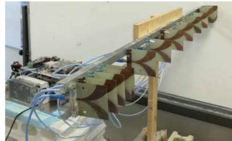
Fig. 5. 1-D MIMO GB-SAR array operating at 4-8GHz [3].
