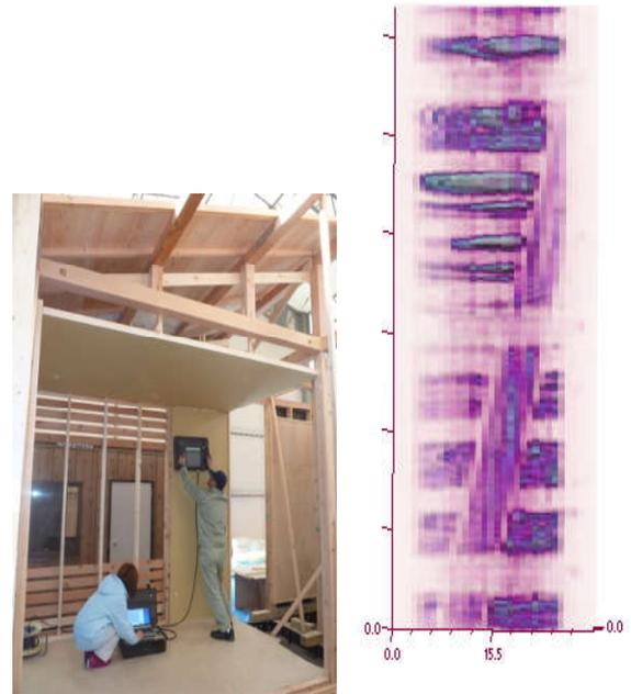
(a) Experiment setup (b) Imaged structure by a 1-D linear array radar.
