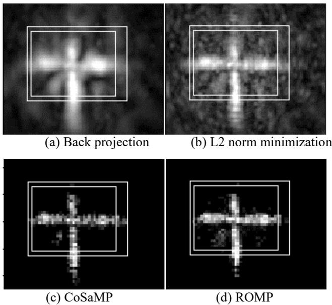
Fig. 11. The reconstructed image of the wooden cross target.
