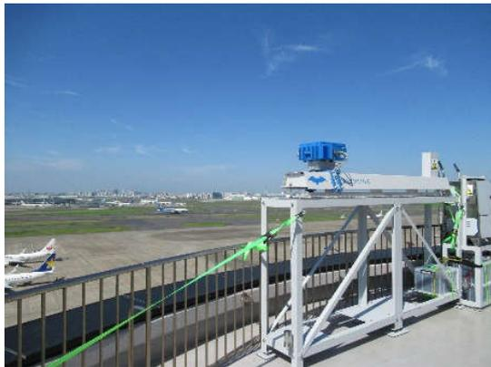
Fig. 3. GB-SAR system installed at Tokyo International Airport (Haneda).
