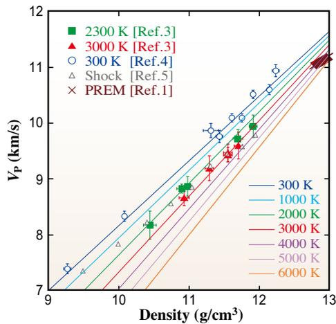
Fig. 2. Compressional velocity of hcp-Fe at several temperatures as a function of density along with high-temperature data [3] and room-temperature data [4] based on IXS and shock compression experiments [5]. Isothermal  $\rho$ - $V_p$  fitting lines are expressed as  $V_p = [1.160\rho - 3.43] + [7.2 \times 10^{-5} \times (T - 300) \times (\rho - 14.2)]$ .
