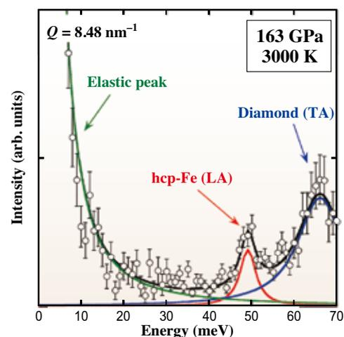
Fig. 1. IXS spectrum of hcp-Fe at 163 GPa and 3000 K. The peak at zero energy is from elastic scattering. Curves are individual contributions (green: elastic scattering, red: LA phonons of hcp-Fe, blue: TA phonons of diamond), with the experimental data fitted with Lorentzian functions.
