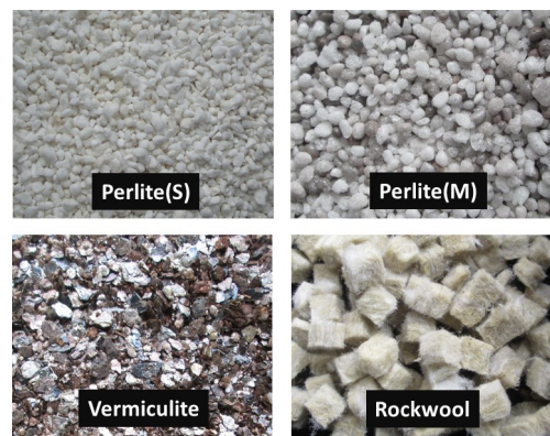
Fig. 2 Four types of solid medium used for the cultivation test of sweetpotato
