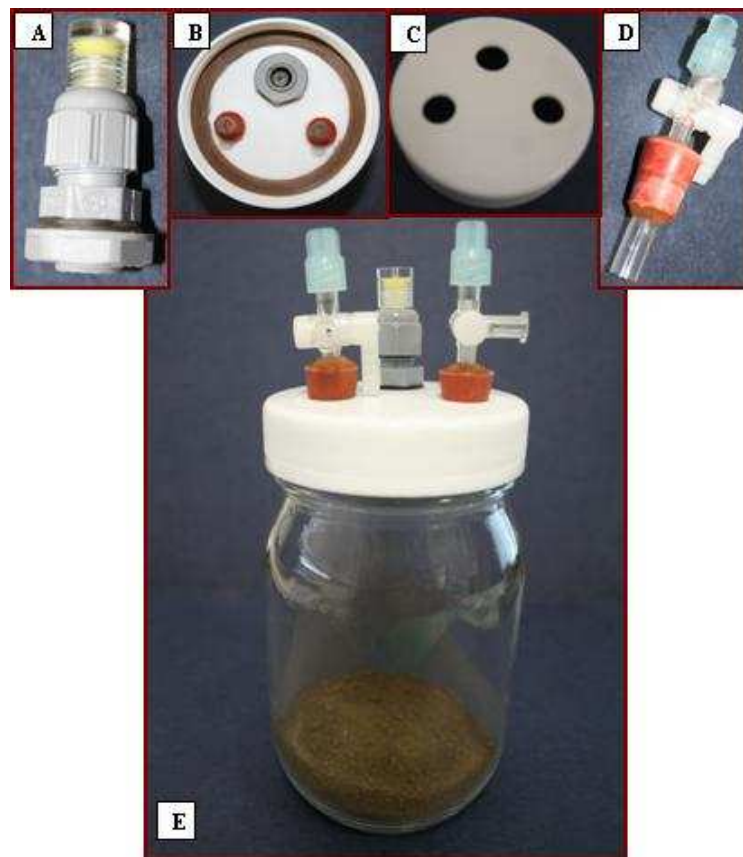
Figure 1. The experimental unit. Acrylic tubing fitted with a septum mounted on cable grand served as the gas sampling port (A); Viewed from the bottom of the lid are the gas sampling port,
