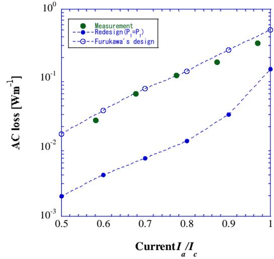
Fig. 10 AC loss characteristics by quasi three-dimensional electromagnetic field analysis.
