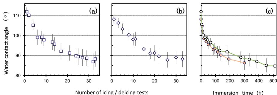
Fig. 3 Evolution of water CA values for (a) FAS and (b) SA coated samples over icing/deicing tests. (c) CA values for FAS (open symbols) and SA (solid symbols) coated samples as a function of immersion time (in DI water). Lines are only given as a guide to the eye.
