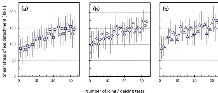
Fig. 2 Shear stress of ice detachment as a function of icing/deicing cycles on (a) FAS, (b) SA and (c) ODTMS-treated surfaces.
