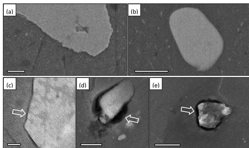
Fig. 1 SEM surface images of polished AA2024 sample coated with FAS: (a and b) after twelve months in air and (c–e) after 33 icing/deicing events. Irregular (a and c) and regular (b, d and e) intermetallic particles and their vicinities are shown. Scale-bars indicate  $1 \mu\text{m}$ . Trenches electrochemically formed between the particles and the surrounding Al matrix are indicated by arrows.
