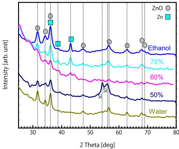
**Fig. 1.** (Color online) XRD patterns of samples prepared via ablation of metal Zn in water-ethanol mixtures at 1 atm (with ethanol concentration of 0, 50, 60, 75, and 99.5 vol %, from bottom to top). The peaks at  $\sim 54^\circ$  are from Si substrates, while the other peaks were indexed as those of wurtzite ZnO (gray circles) or metallic Zn (blue squares).
