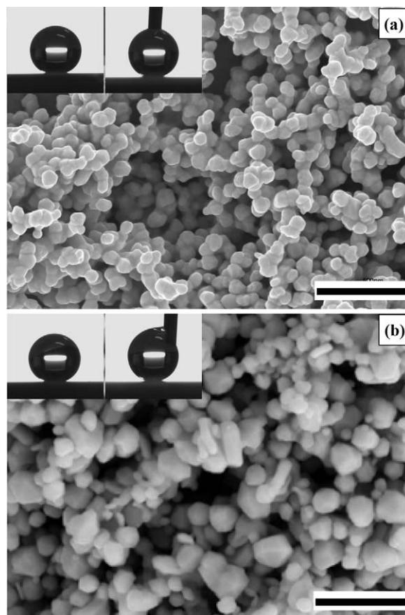
Fig. 4. SEM images of samples 5(a) and 6(b) prepared from Ag nanoparticles. Sessile and moving water droplets are shown as insets. Scale bars indicate 1  $\mu$ m.
