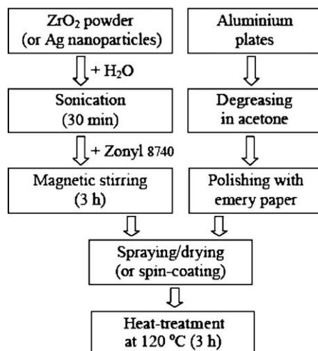
**Fig. 1.** Schematic representation of coating procedure.
