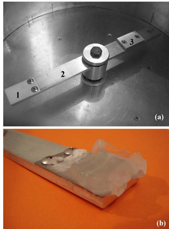
**Fig. 2.** (a) Coated sample in centrifuge set-up measuring ice adhesion: (1) sample, (2) Al beam and (3) counter-weight. (b) Sample with artificial glaze ice.
