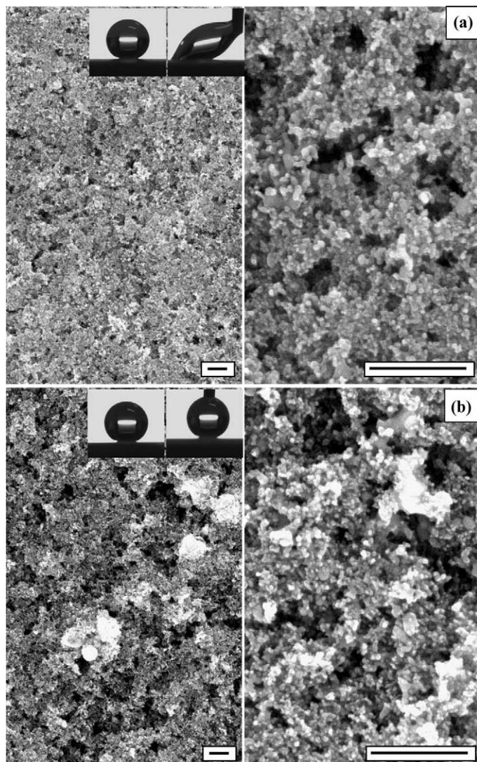
Fig. 3. Surface images of samples 3(a) and 4(b) prepared from  $ZrO_2$  nanopowder. Sessile and moving water droplets are shown as insets. Scale bars indicate 500 nm.
