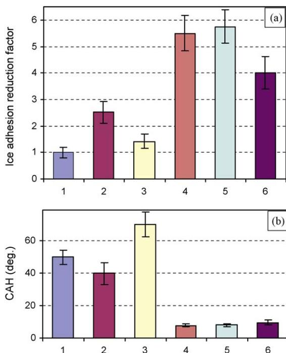
Fig. 6. Values of ice adhesion reduction factor (ARF) (a) and contact angle hysteresis (b) for samples used. Sample numbers correspond to Table 1.
