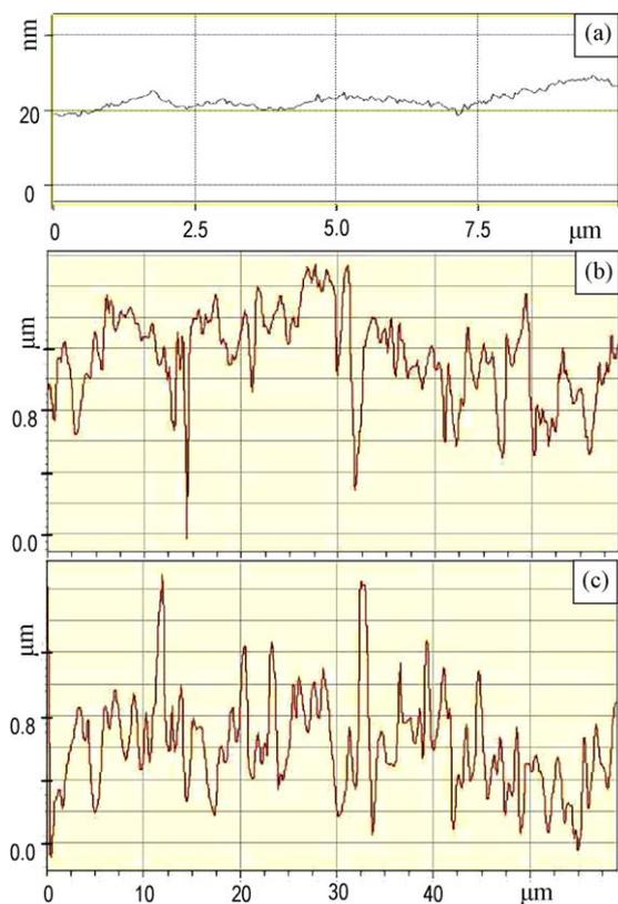
Fig. 5. Surface profiles of samples 2(a), 3(b) and 4(c).
