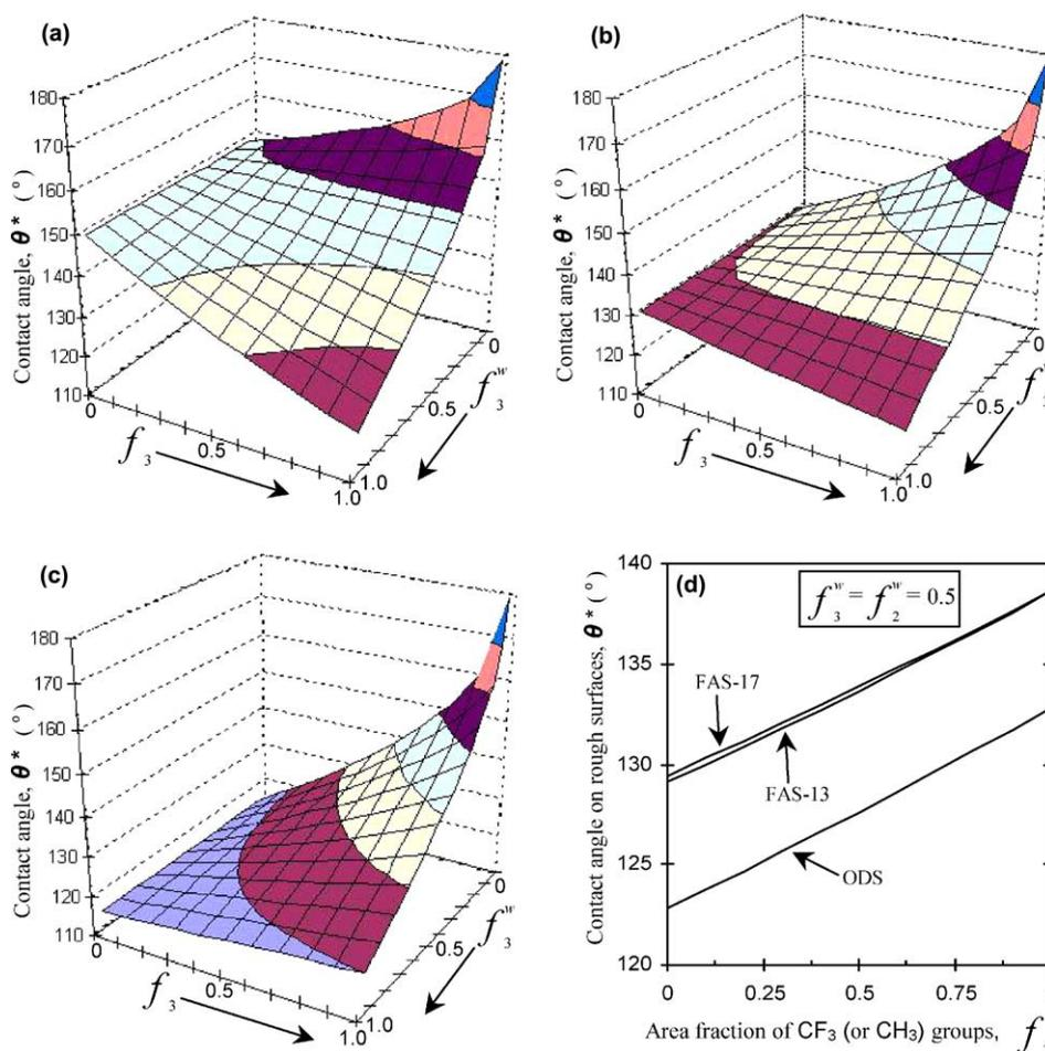
Fig. 4. (a)–(c) Contact angle of FAS-17-grafted rough “composite” surfaces as a function of SAM assembly order ( $f_3$ ) and water coverage of  $\text{CF}_3$ -terminated patches ( $f_3^w$ ). The water coverage of  $\text{CF}_2$  ( $\text{CH}_2$ )-terminated patches ( $f_2^w$ ) equals 0.2 (a); 0.5 (b); and 0.8 (c). (d) Comparison of wetting behavior of FAS-17, FAS-13, and ODS-grafted rough “composite” surfaces as a function of  $f_3$  under water-coverage regime of  $f_3^w = f_2^w = 0.5$ .
