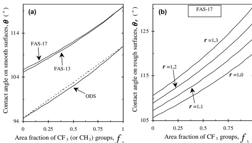
Fig. 3. Contact angle of water droplet on SAM-grafted surfaces as a function of assembly order/disorder degree. (a) Smooth surfaces with 1H,1H,2H,2H-perfluorodecylsiloxane (FAS-17), 1H,1H,2H,2H-perfluorooctylsiloxane (FAS-13), and octadecylsiloxane (ODS) monolayers. Dashed and solid lines indicate surfaces with micro-sized and nano-sized heterogeneous patches, respectively. (b) Effect of roughness for FAS-17 monolayers in Wenzel's wetting regime. Curves for nano-patches are presented.
