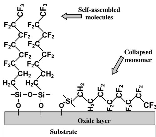
Fig. 1. 1H,1H,2H,2H-perfluorooctylsiloxane (FAS-13) monolayer on an oxide surface. Well-oriented, or self-assembled, (left) and collapsed (right) molecules are shown, exposing their topmost  $\text{CF}_3$  and  $\text{CF}_2$  (or  $\text{CH}_2$ ) groups, respectively.
