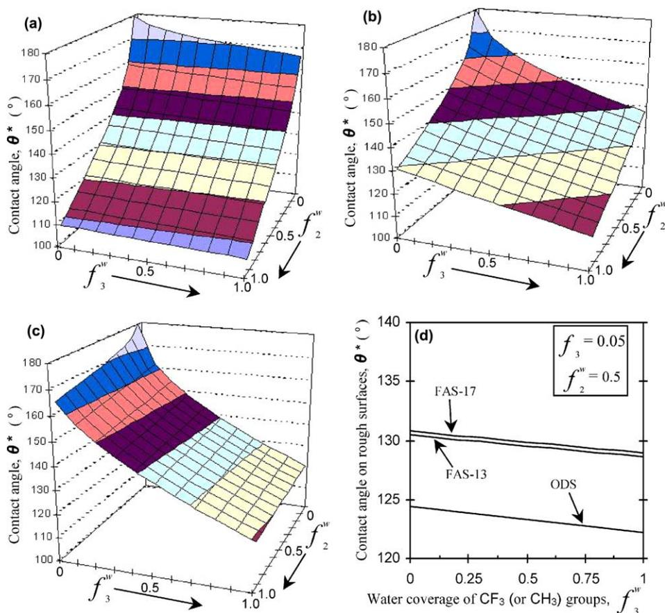
Fig. 5. (a)–(c) Contact angle of FAS-17-grafted rough “composite” surfaces as a function of water coverage of  $\text{CF}_3$ -terminated patches ( $f_3^w$ ) and  $\text{CF}_2$  ( $\text{CH}_2$ )-terminated patches ( $f_2^w$ ). The self-assembly order ( $f_3$ ) equals 0.05 (a); 0.5 (b); and 0.95 (c). (d) Comparison of wetting behavior of FAS-17, FAS-13, and ODS-grafted rough “composite” surfaces as a function of  $f_3^w$  at  $f_2^w = 0.5$  and  $f_3 = 0.05$ .
