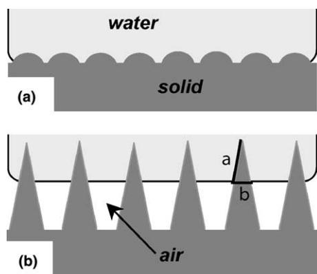
Fig. 2. (a) Schematic representation of wetting of hydrophobic solid surface at low roughness. (b) Air is entrapped beneath the water droplet on the surface after certain increase in roughness. Schematic illustration of the model surface composed of a series of uniform needles which is used for sliding angle calculations.
