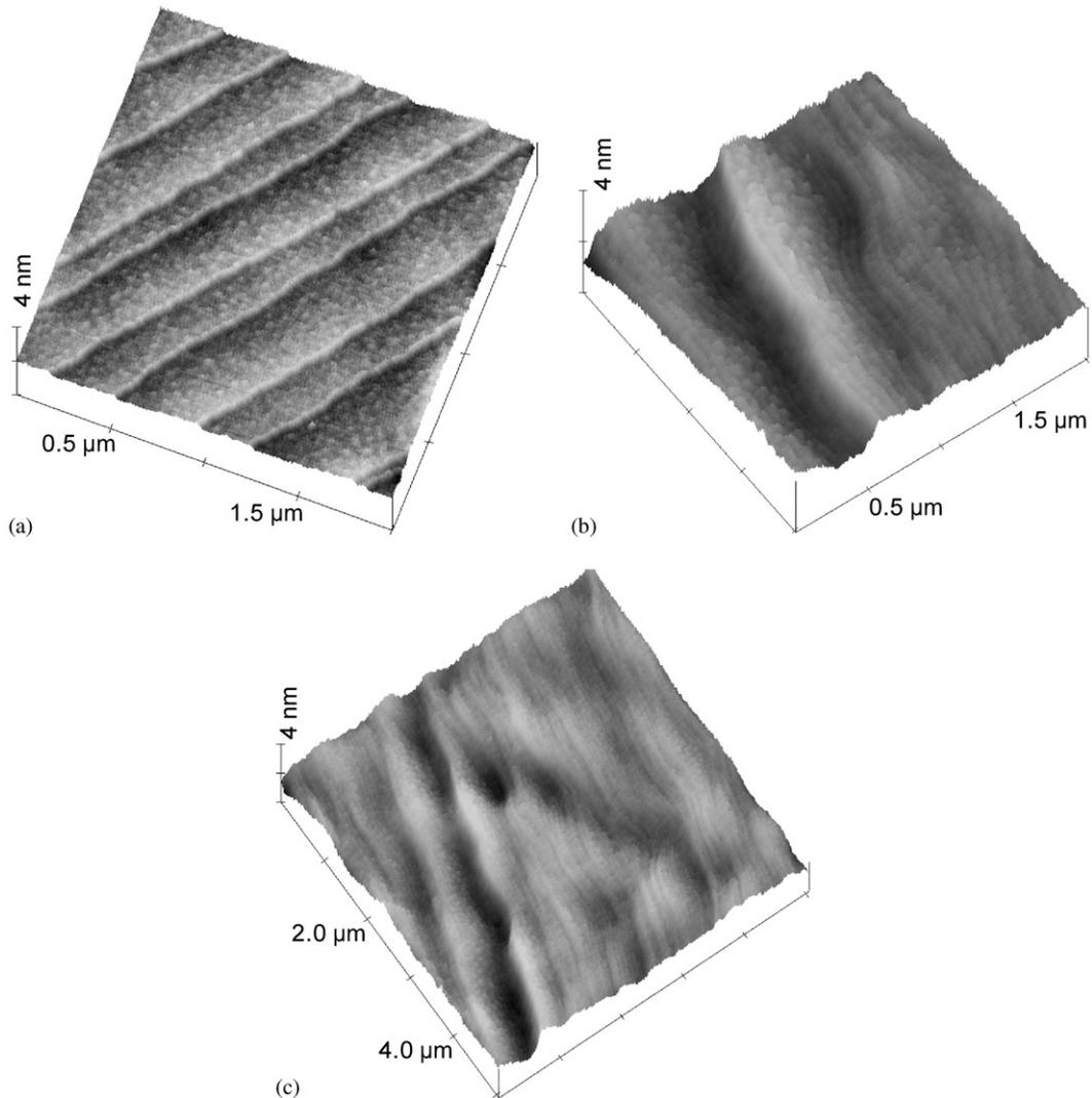
Fig. 8. AFM surface images of the LN (a) and LT (b,c) substrates heat-treated at 1000°C for 1 h in air. Surface areas of  $2 \times 2 \mu\text{m}^2$  (a,b) and  $5 \times 5 \mu\text{m}^2$  (c) are shown.
