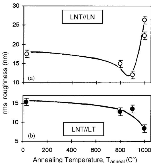
Fig. 7. LNT film root-mean-square roughness as a function of LN (a) and LT (b) substrate pre-deposition annealing temperature in air. All the films, 180–200 nm thick, were grown at  $T_{\text{sub}} = 650 \pm 10^{\circ}\text{C}$  and 180–200 nm/min. Solid lines are added only as visual guides.
