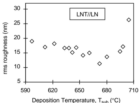
Fig. 4. Film root-mean-square roughness as a function of average deposition temperature for 180–200-nm-thick LNT films deposited at 180–200 nm/min on as-received (001)LN wafers.
