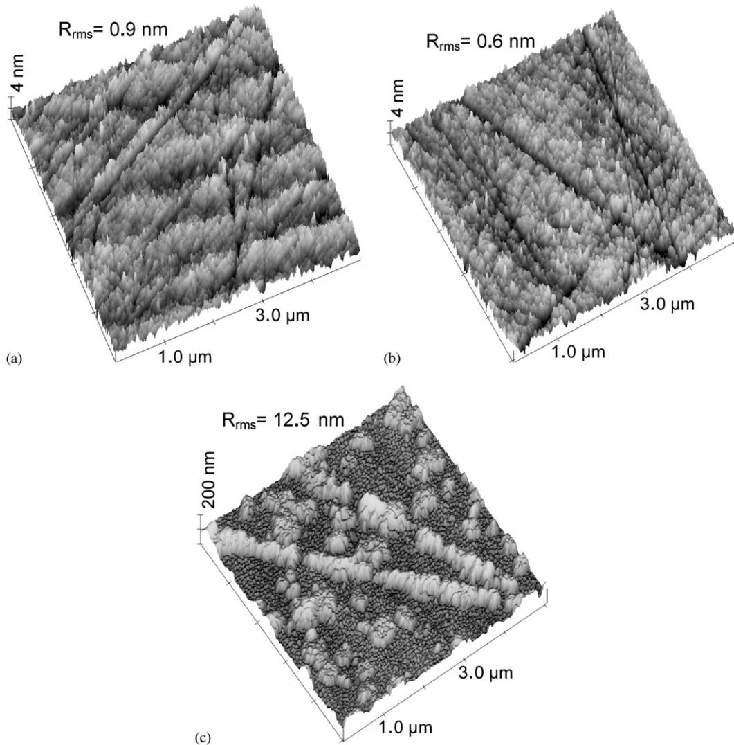
Fig. 6. AFM surface images ( $5 \times 5 \mu\text{m}^2$ ) of the as-received LT (a) and LN (b) substrates. Numerous nano-scratches and corrugations of the surfaces are seen. (c) AFM surface image ( $5 \times 5 \mu\text{m}^2$ ) of the LNT film deposited on as-received LT substrate at 100 nm/min and  $T_{\text{sub}} = 595 \pm 10^\circ\text{C}$  for 1 min. Rows of high islands formed along substrate surface scratches are clearly seen.
