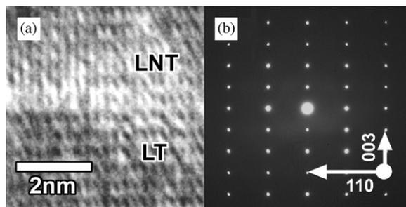
Fig. 2. (a) Cross-sectional HRTEM image of the 100-nm-thick LNT film on as-received LT grown at 100 nm/min and  $T_{\text{sub}} = 595 \pm 5^\circ\text{C}$ . (b) SAED pattern of the LNT//LT interface for the same sample. The zone axis is  $[\bar{1} 1 0]$ .
