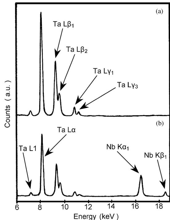
Fig. 1. EDS spectra of the 100-nm-thick LNT film on as-received LT grown at 100 nm/min and  $T_{\text{sub}} = 595 \pm 5^\circ\text{C}$ : (a) LT substrate area, (b) LNT film area.
