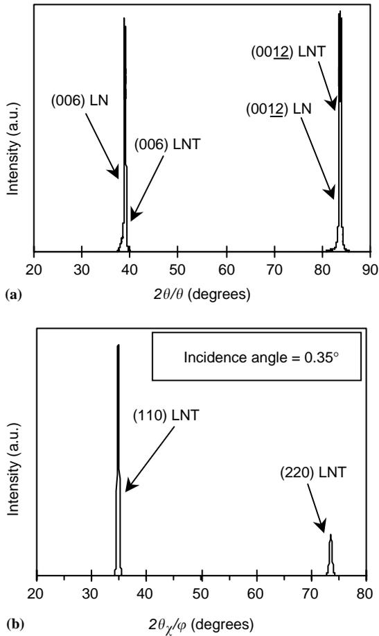
Fig. 3. XRD  $2\theta/\theta$  scan pattern (a) and in-plane  $2\theta\gamma/\phi$  scan pattern (b) of the 190-nm-thick  $\text{LiNb}_{0.5}\text{Ta}_{0.5}\text{O}_3$  film on as-received LN substrate, deposited at 50 nm/min and  $T_{\text{sub}} = 625 \pm 5^\circ\text{C}$ . The incidence angle used for (b) was  $0.35^\circ$ .
