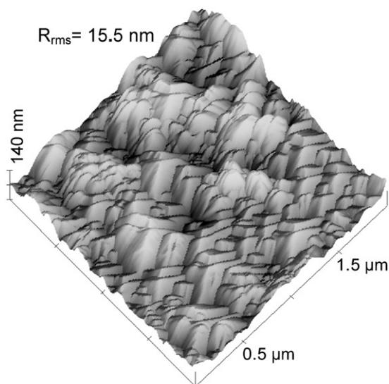
Fig. 5. AFM surface image ( $2 \times 2 \mu\text{m}^2$ ) of LNT film on as-received LN substrate grown at 50 nm/min and  $T_{\text{sub}} = 695 \pm 5^\circ\text{C}$  for 4 min. Three-fold symmetry of the surface-forming islands is revealed.
