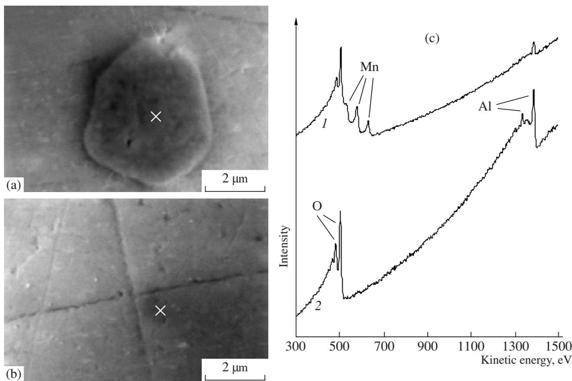
**Fig. 2.** SEM micrographs of (a) an Al–Cu–Mg particle and (b) the alloy matrix on the surface of an AA2024 sample treated at room temperature for 1 min; (c) local Auger electron spectra of the regions marked in panels (1) a and (2) b.
