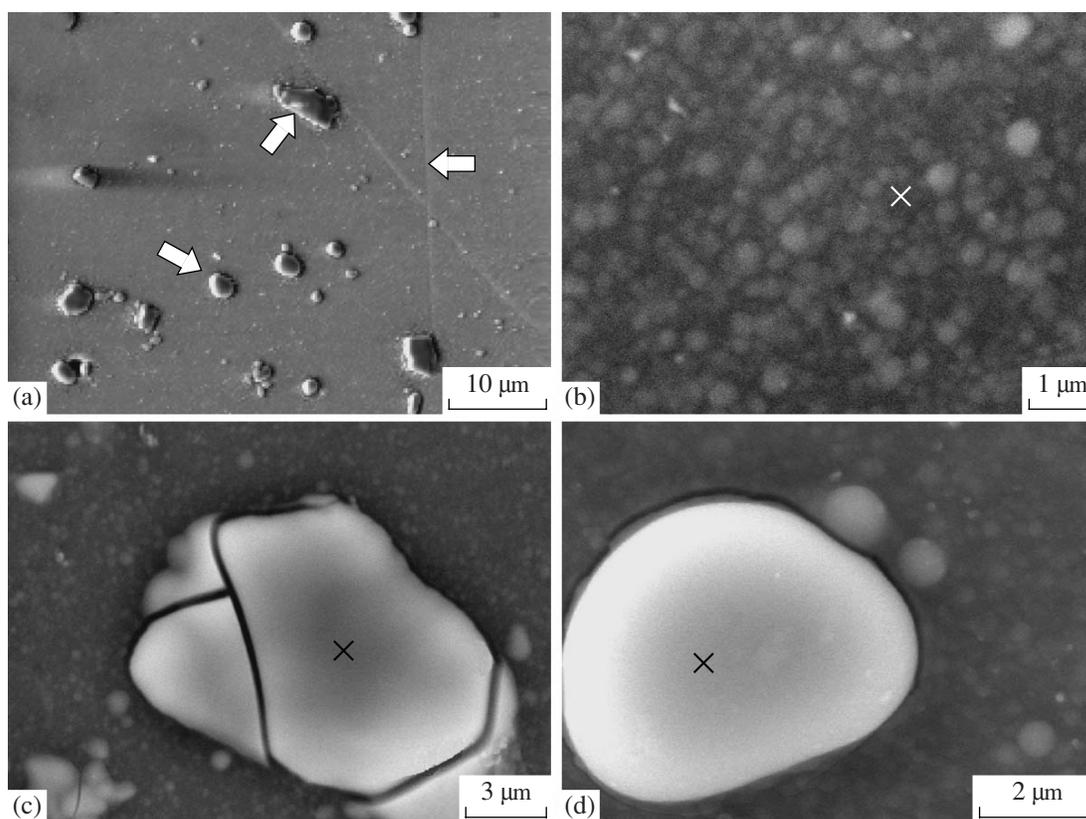
**Fig. 4.** SEM micrographs of AA2024 samples treated at room temperature for (a) 30 and (b–d) 150 min; (a) well-coated Al–Cu–Mg particles (smaller) and Al–Cu–Fe–Mn particles (larger); the arrow at the right of the micrograph marks a polishing scratch; (b) evenly coated matrix; (c) Al–Cu–Fe–Mn and (d) Al–Cu–Mg particles with thick PCCs.
