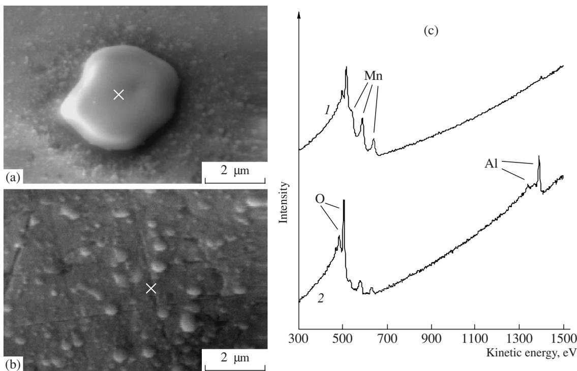
**Fig. 3.** SEM micrographs of (a) an Al–Cu–Mg particle and (b) the alloy matrix on the surface of an AA2024 sample treated for 20 min; (c) local Auger electron spectra of the regions marked in panels (1) a and (2) b.
