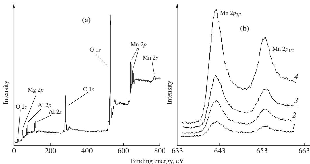
**Fig. 1.** (a) XPS survey scan of AA2024 treated at room temperature for 60 min; (b) Mn 2p spectra of samples treated for (1) 5, (2) 20, (3) 60, and (4) 150 min.
