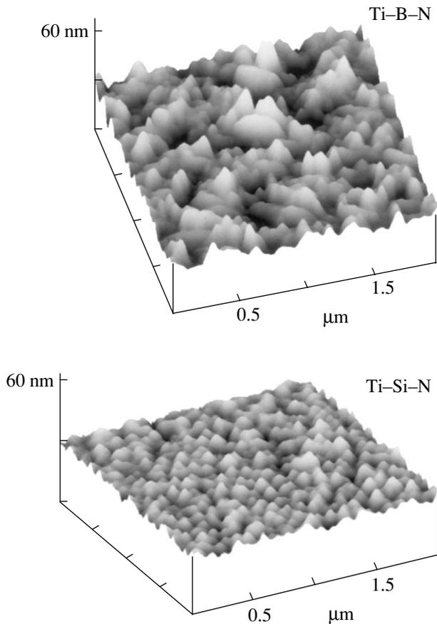
**Fig. 1.** Surface topography of Ti-B-N (2) and Ti-Si-N films.
