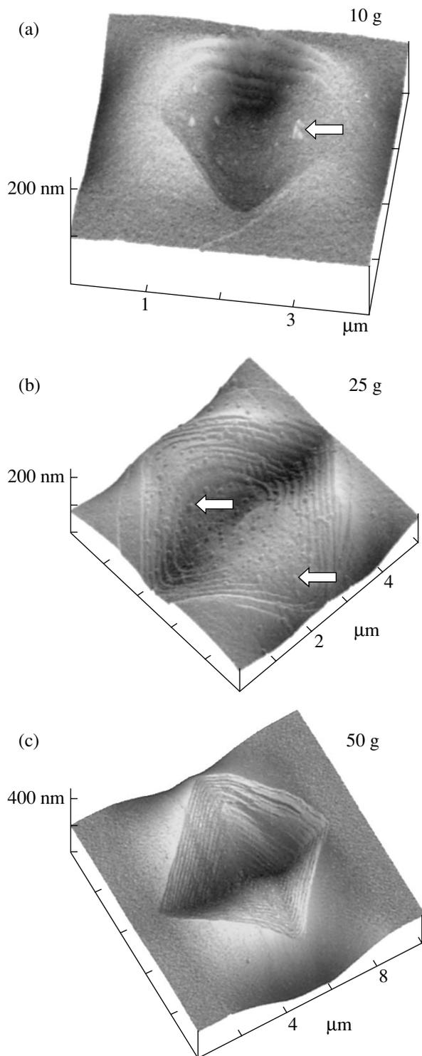
**Fig. 6.** AFM images of regions with localized deformation in a Ti-Cr-B-N film indented with a Vickers pyramid at a load of (a) 10, (b) 25, and (c) 50 g. Particles rejected outside are shown by arrows.
