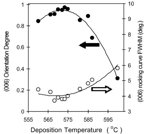
Fig. 3. Variation of orientation degree ( $f$ ) for  $\text{LiNb}_{0.5}\text{Ta}_{0.5}\text{O}_3$  (160–180 nm thick) films as a function of deposition temperature  $T_{\text{sub}}$  (the change of the (0 0 6) rocking-curve FWHM value for the same films is also shown).
