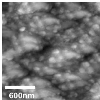
Fig. 6. Surface morphology of the 170 nm thick LiNb<sub>0.5</sub>Ta<sub>0.5</sub>O<sub>3</sub> film deposited at *R* = 4 ml/min for 1 min onto Si(1 0 0) substrate with previously formed 900 nm thick SiO<sub>2</sub> buffer layer. *T*<sub>sub</sub> = 570°C; (0 0 6) rocking curve FWHM value 4.2°; rms roughness 14 nm.
