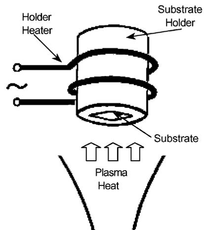
Fig. 1. Scheme of the improved substrate heating system of the TPS CVD apparatus depicting independent holder heating by both auxiliary Cu inductive coil and plasma with fixed power.
