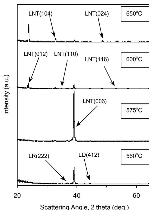
Fig. 2. Variation of XRD patterns of  $\text{LiNb}_{0.5}\text{Ta}_{0.5}\text{O}_3$  films deposited on SiO<sub>2</sub>/Si (oxide thickness about 900 nm) substrates with deposition temperature  $T_{\text{sub}}$ .
