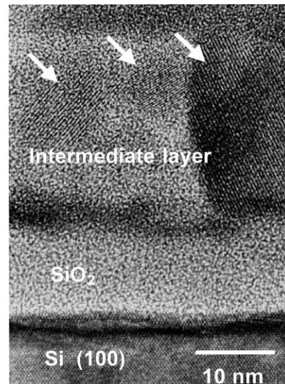
Fig. 5. A cross-sectional HR TEM image for the  $\text{LiNb}_{0.5}\text{Ta}_{0.5}\text{O}_3$  film deposited onto a Si(1 0 0) substrate with a native  $\text{SiO}_2$  layer. Only interface areas including Si,  $\text{SiO}_2$  and the amorphous intermediate layer of approximately 30 nm are shown. One large and two smaller LNT crystallites within the latter are depicted with white arrows.
