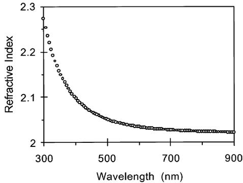
Fig. 7. Refractive index for a 300 nm thick  $\text{LiNb}_{0.5}\text{Ta}_{0.5}\text{O}_3$  film deposited onto a  $\text{SiO}_2/\text{Si}(111)$  substrate (oxide thickness about 700 nm) at  $R = 8$  ml/min, measured by spectroscopic ellipsometry.
