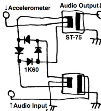
Figure 8: Ring modulation circuit
