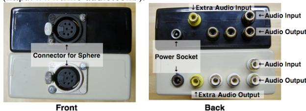
Figure 6: Converter boxes (Black for the sphere with the transmitter, White for the sphere with the receiver)
