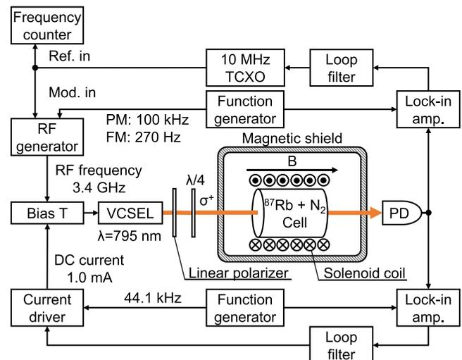
FIG. 2. Schematic diagram of the atomic clock used in the experiment. PD: photodetector and TCXO: temperature-compensated crystal oscillator.
