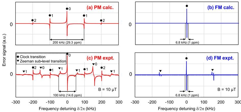
FIG. 3. Error signals with PM and FM: (a) calculation result with PM when a bias magnetic field of  $10 \mu\text{T}$  is applied, (b) calculation result with FM, (c) experimental result with PM, and (d) experimental result with FM when a bias magnetic field of  $10 \mu\text{T}$  is applied.
