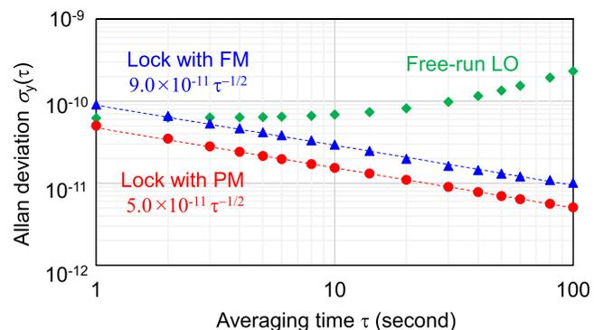
FIG. 4. Allan deviations: the circular and triangular dots are those for the CPT atomic clock with PM and FM, respectively. The square dots are those for free-run LO.
