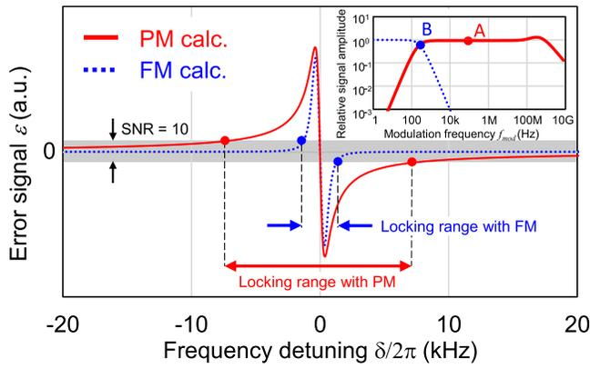
FIG. 1. Numerically calculated error signal of CPT resonance with PM (red solid line) and FM (blue dot line): The gray band shows the noise level in the case of SNR = 10, which determines locking ranges. The inset shows the signal amplitude as a function of modulation frequency. Points A and B for PM and FM are the operating points that we employed in this work. The full width at half maximum of the CPT resonance  $\gamma/\pi$  is set at 540 Hz.
