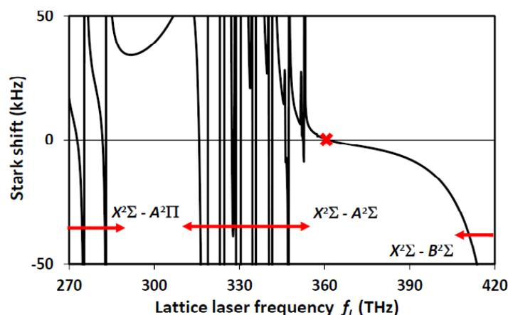
**Fig 1.** The Stark shift in the  $^{174}\text{Yb}^6\text{Li}$  ( $v,N$ ) = (0,0)-(1,0) transition frequency induced by the trap laser frequency with the power density of 23 kW/cm<sup>2</sup> as a function of trap laser frequency  $f_L$ . The magic trap frequency, listed in Table 2, is highlighted [(red crosses)]. The (red) arrows denote the frequency region that is quasi-resonant with the  $X^2\Sigma$ ,  $A^2\Pi$ ,  $A^2\Sigma$ , and  $B^2\Sigma$  transitions.
