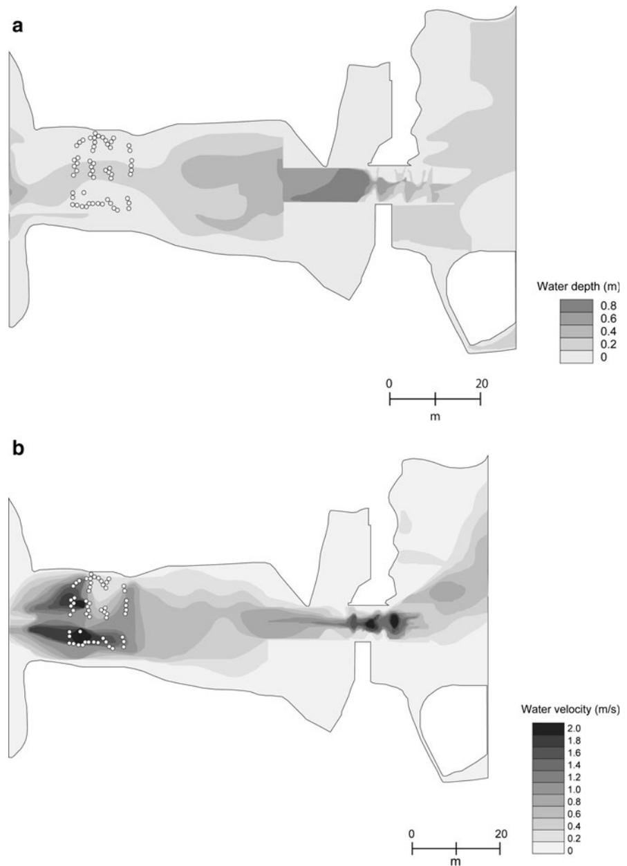
Water velocity in the migration paths through the protection bed of #5 ground sill tended to be higher for unsuccessful fish (Fig. 4b) than those for successful fish (Fig. 4a). Table 3 shows that water velocity and water depth in the migration paths at the protection bed of #5 ground sill and the fishway of #6,7 ground sill in all successful and unsuccessful fish, respectively. Water velocity was significantly higher for unsuccessful fish than for successful fish,
