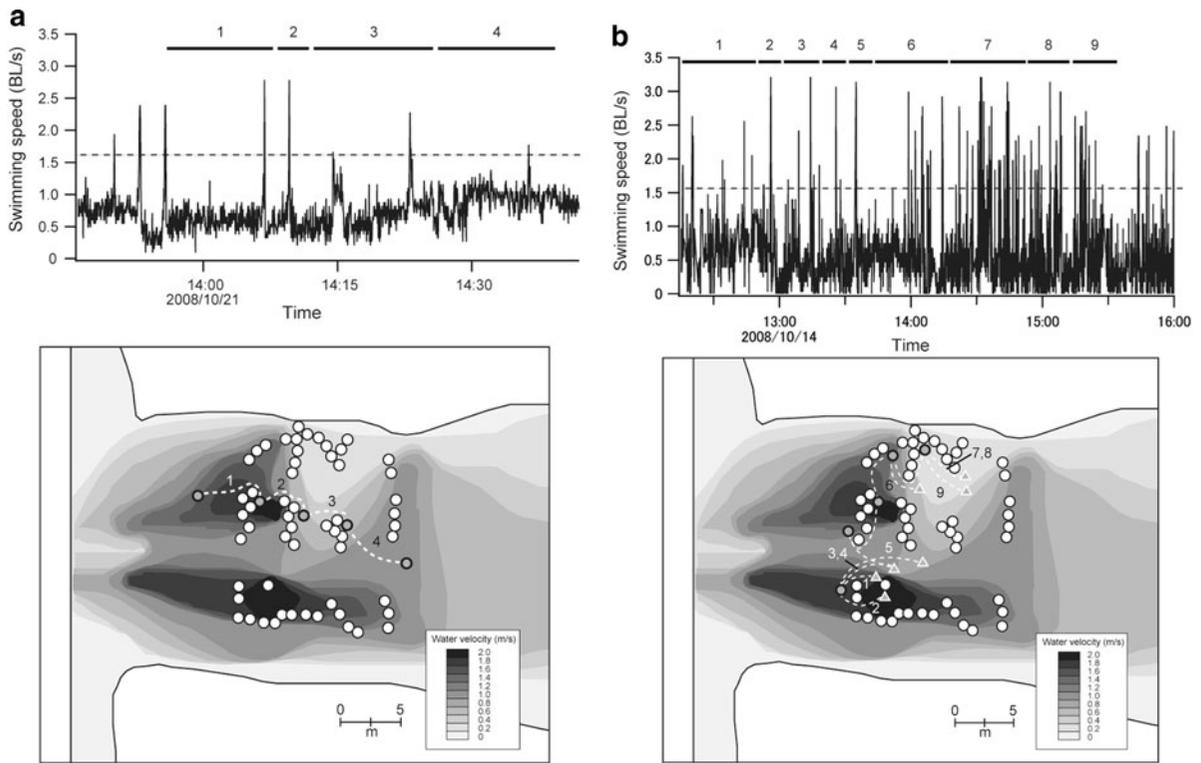
**Fig. 4** Time-series plots of swimming speeds of successful (a) and unsuccessful (b) chum salmon and dotted line represent a mean critical swimming speed (1.55 BL/s) (upper figure). Swimming path (white dotted line) of successful (a) and
