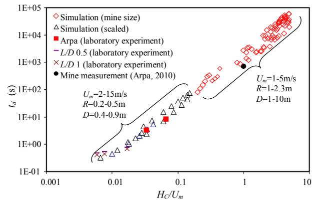
Figure 6. Relationship between average time delay,  $t_d$ , and dead space ratio
