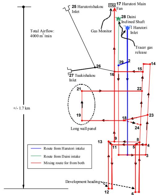
Figure 8. Kushiro Coal Mine's ventilation network (2011)
