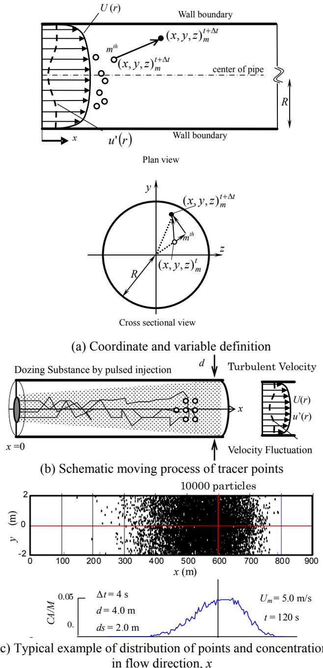
Figure 2. Schematic definitions of tracer point movements in ( $x$ - $y$ ) and ( $y$ - $z$ ) cross sections.
