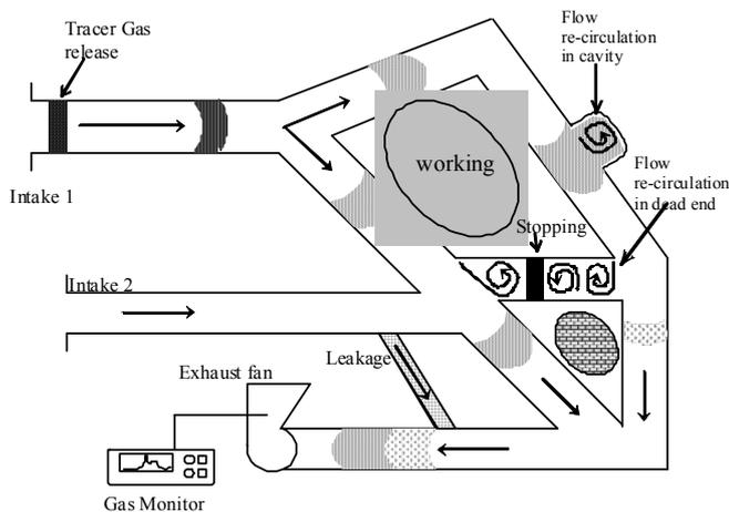
Figure 1. Illustration of tracer gas measurement in underground mine ventilation network
