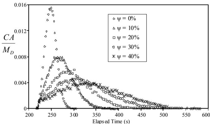
Figure 7. Simulation results using DTPM for different dead space ratio,  $\psi$  (%) for  $U_m = 2$  m/s,  $d=3$ m.
