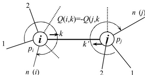
Figure 3. Definitions of airways connection and variables for network flows (Sasaki & Dindiwe, 2002)
