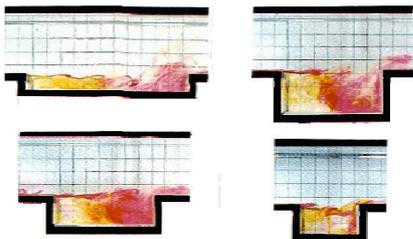
Figure 4. Schematic depiction of the laboratory testing to measure decay time of gas in a cavity
