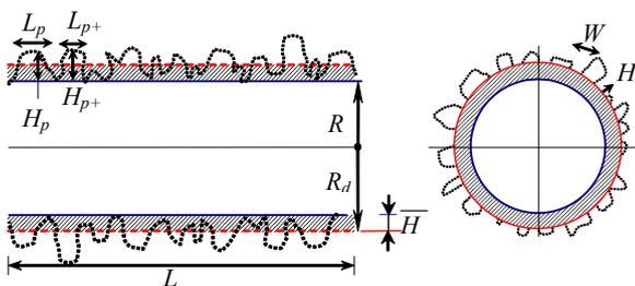
Figure 5. Simplified model of small cavities distributed around circular airways that is treated as extended region of airways
