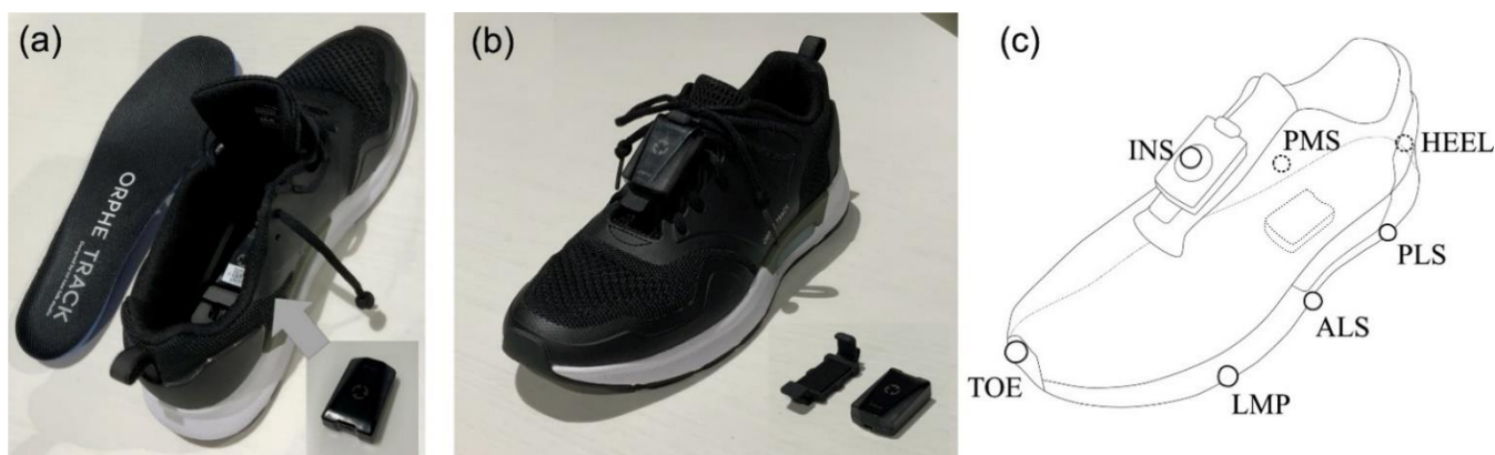
Figure 1. (a) Motion sensor embedded in the shoe midsole; (b) Motion sensor mounted on the shoe instep with dedicated mounting equipment; (c) Marker position on the shoe. (a) The shoe has space for sensor placement, and the center of the sensor is located 40% of the shoe's length from the heel edge. (b) A motion sensor mounted on the shoe instep using dedicated mounting equipment that can be fixed to the shoelace. (c) The names and position definitions of the reflective markers are as follows: LMP, the lateral edge of the metatarsophalangeal joint; TOE, the most anterior edge of the shoe; PLS, the posterior lateral side of motion sensor; ALS, the anterior lateral side of motion sensor; PMS, the posterior medial side of motion sensor; HEEL, the most posterior edge of the shoe midsole; INS, the center of the sensor mounted on the instep equipment of the shoe.
