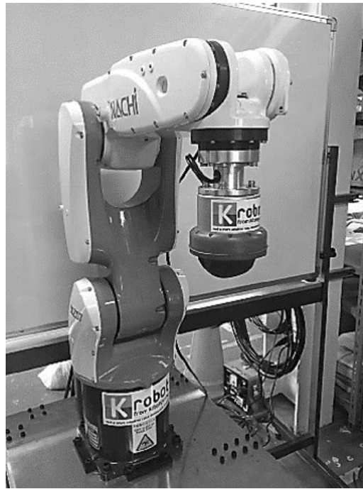
Fig. 9. Six-axes industrial robot equipped with developed novel gripper using MR \alpha fluid.
