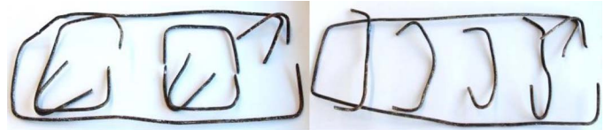
Fig. 11. Damage to hoop and crosstie confinement in the localized failure regions of A10.
