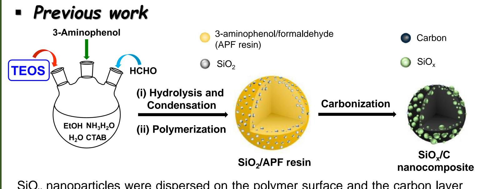
SiO<sub>x</sub> nanoparticles were dispersed on the polymer surface and the carbon layer did not perfectly coat  $SiO_x$ , leading to a low reversible capacity.
