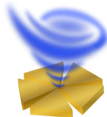
Figure 1: Nano-shaping of photons. Conceptual illustration of plasmonic nano-vortex fields formed by metal multimer structures, where the orbital angular momentum (OAM) and spin angular momentum (SAM) are transferred from Laguerre–Gaussian (LG)-mode beams to localized plasmons and then confined into nanometer-sized gaps.
