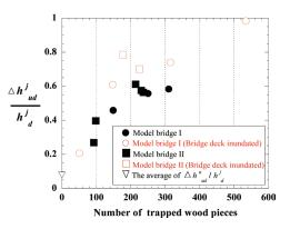
Figure 16. Relationship between the normalized backwater rise and the number of wood pieces trapped by a model bridge.
