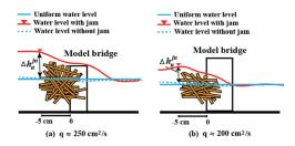
Figure 15. A schematic feature of backwater rise.
