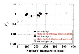
Figure 18. Relationship between the loss coefficient and the number of trapped wood pieces.
