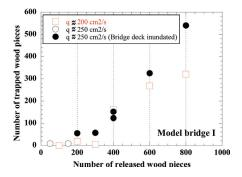
Figure 7. The number of wood pieces trapped by the model bridge I during water flow.
