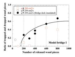
Figure 9. The number ratio of wood pieces trapped by model bridge I and dropped at the station 'd' during water flow.
