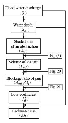
Figure 22. A flow chart for predicting backwater rise.
