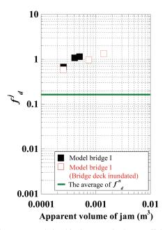
Figure 19. Relationship between the loss coefficient and the apparent volume of log jam at a model bridge.
