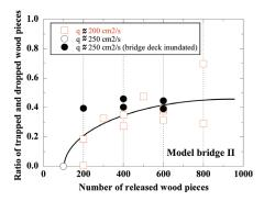
Figure 10. The number ratio of wood pieces trapped by model bridge II and dropped at the station 'd' during water flow.
