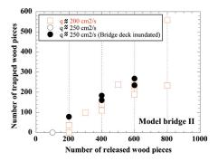
Figure 8. The number of wood pieces trapped by the model bridge II during water flow.
