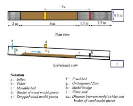
Figure 1. Experimental flume.
