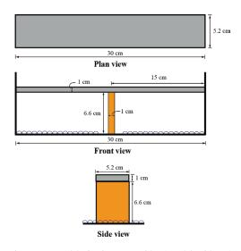
Figure 3. Model of Miyanoue Bridge (Model Bridge II).
