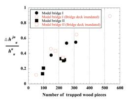
Figure 17. Relationship between the normalized backwater rise and the number of wood pieces trapped by a model bridge.
