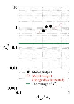
Figure 21. Relationship between the loss coefficient and the blockage ratio of jam.
