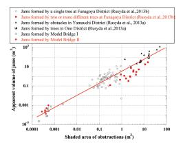
Figure 12. Volume of log jams versus shaded area of obstructions in real river and laboratory flume.
