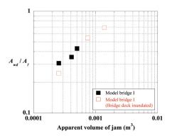
Figure 20. Relationship between the blockage ratio of jam and apparent volume of log jam at a model bridge.
