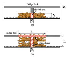
Figure 11. The definition of the 'shaded area' of an obstruction, such as the case of a jam formed by a pier (a) and that of a jam formed by bridge deck and pier.
