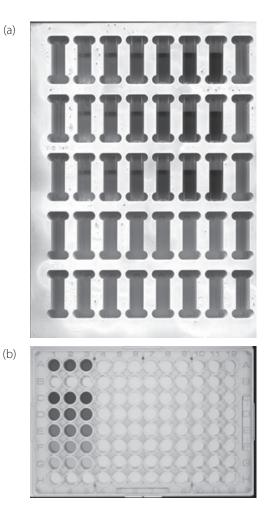
Figure 9: Digital image obtained from FC method (a) GT-S620 image of FC-treated CA. (b) D70s image of CA (1-C to G, 2-C to G, 3-C to G), and unknown concentration samples (1-A, 2-A, 3-A). Micro-plate was placed on a flat LED light panel.
