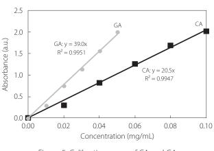
Figure 5: Calibration curve of CA and GA
