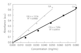
Figure 8: Calibration curve of CA and GA using digital camera (Nikon D70s)
