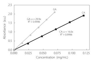
Figure 7: Calibration curve of CA and GA using micro-plate reader (ChroMate 4300)
