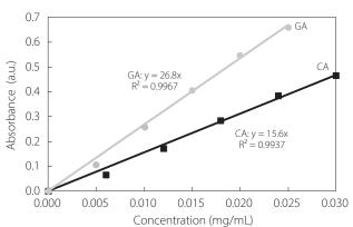
Figure 6: Calibration curve of CA and GA using the scanner (EPSON GT-S620)
