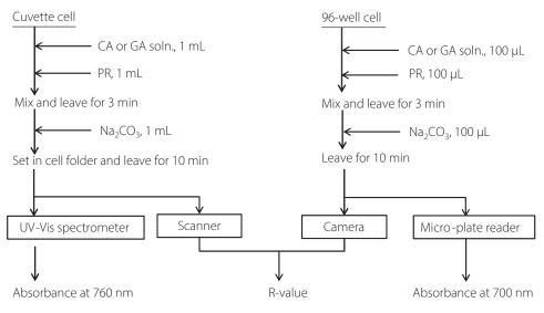
Figure 2: Experimental procedure
