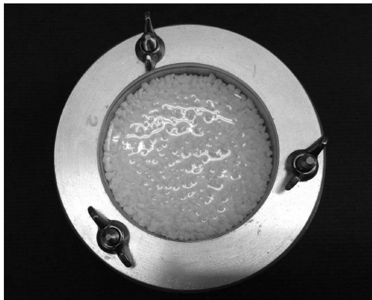
Fig. 2. Top view photograph of the PP film on a conventional screw-type cup after measuring WVTR at 85 °C.
