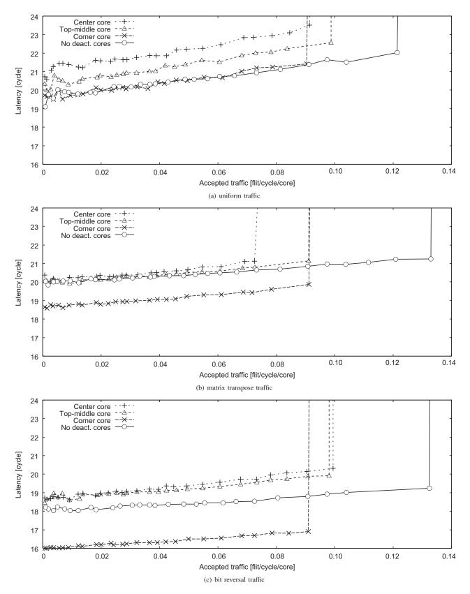
Fig. 4. Accepted traffic vs. latency for 2-D Mesh of 9 cores
