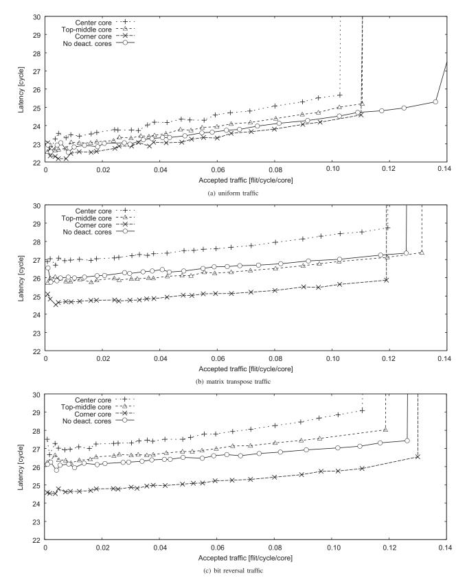
Fig. 5. Accepted traffic vs. latency for 2-D Mesh of 16 cores
