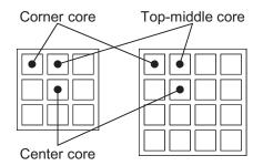
Fig. 3. Patterns of deactivated cores.
