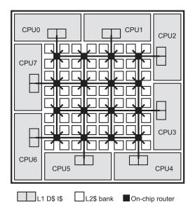
Fig. 1. Example of an 8-core CMP.
