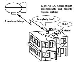
**Figure 5:** The procedure of searching victims by IDC-R
