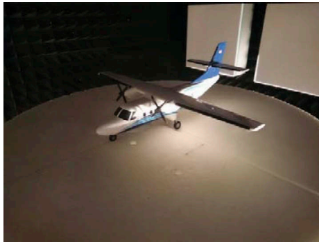
(a) Scattering target used N219 aircraft model
