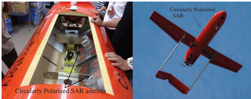
(d) Installed Circularly Polarized SAR antennas and flying test of UAV JX-1 at Fujikawa airfield, Japan
