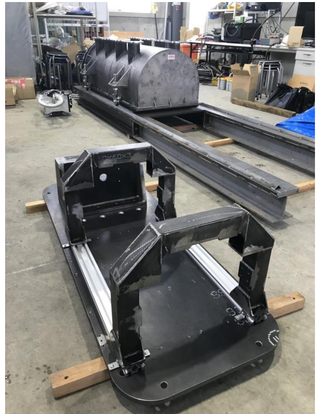
Fig. 15. High altitude simulation chamber under construction for full-scale hybrid rocket thruster testing.
