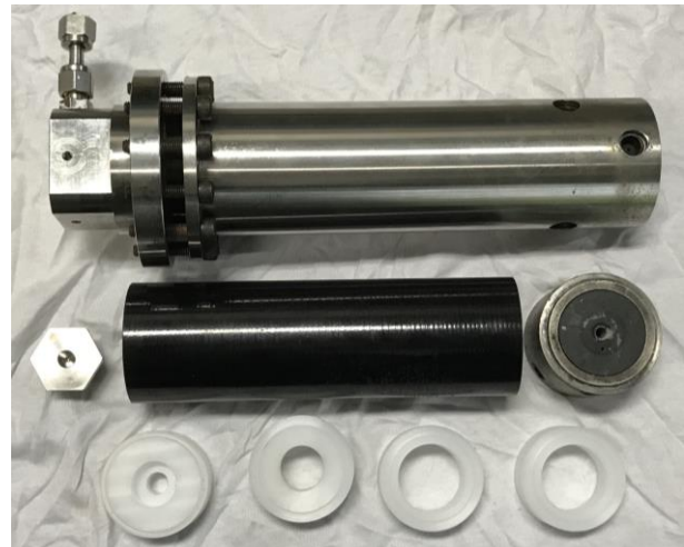
Fig. 1. Sub-scale N_2O /HDPE Test Motor
