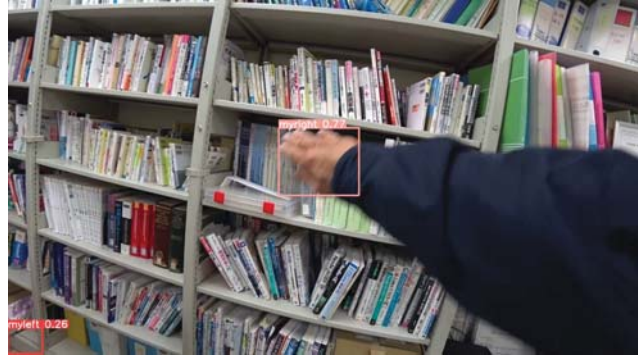
Figure 1: Right hand object detection and recognition using YOLOv5
