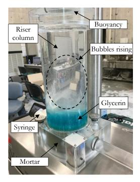
Fig. 5. Measurement of air diameter using air void analyzer.
