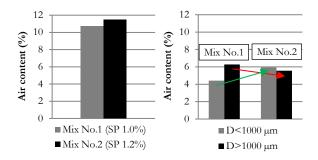
(a) Adjusted air content of concrete, a green arrow indicates air volume increase, a red arrow indicates air volume reduction.
