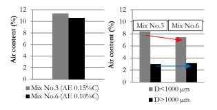
(a) Adjusted air content of concrete, a red arrow indicates air volume reduction, a blue arrow indicates similar air volume.
