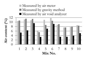
Fig. 6. Initial air content of mix proportions measured using three methods.
