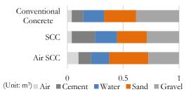
Fig. 1. Volume of materials to make 1 m<sup>3</sup> of concrete.
