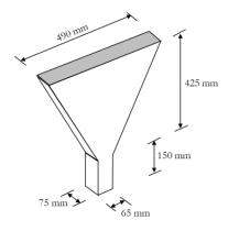
Fig. 4. Standard size of V-funnel for concrete.
