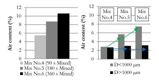
(a) Adjusted air content of concrete, a green arrow indicates air volume increase, a blue arrow indicates similar air volume.
