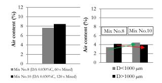
(a) Adjusted air content of concrete, a green arrow indicates air volume increase, a red arrow indicates air volume reduction.
