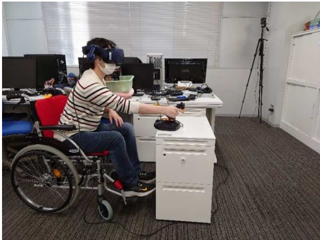
Fig. 1. The manipulating simulator for electric-powered wheelchair utilizing virtual reality technology
